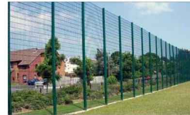
Zaun DU08 perimeter fence system: Height: 6.00m Vertical wires: 6mm Horizontal wires: 8mm Mesh: 200x50mm Post section: 120x60mm Post centres: 2.525m V-beam: included Colour: Green
